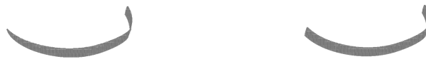
Figure 7: Skeleton of the letter noon requires that the pen rotates to achieve different widths. In the left glyph (correct), the pen inclination from the x-axis changes from 70 to 120 degrees as it moves from right to left. In the right glyph (wrong), the same segment is drawn with a pen of fixed inclination of 75 degrees.
