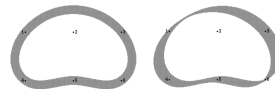
Figure 6: One path traced by two different pens [7]. The left-hand path was drawn using a circular pen, and the right-hand path used an elliptical pen inclined at 40 degrees from the x-axis.
