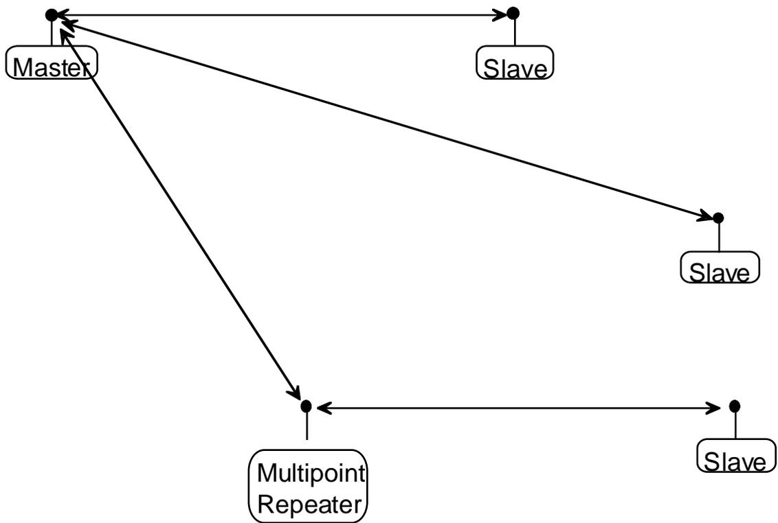
Example (E) depicts a standard point-to-multipoint system. In this example any data sent from the master is broadcast to all three slaves, one of which receives it through a multipoint repeater. The data is in turn sent out of the RS232 port of each of the three slaves.
